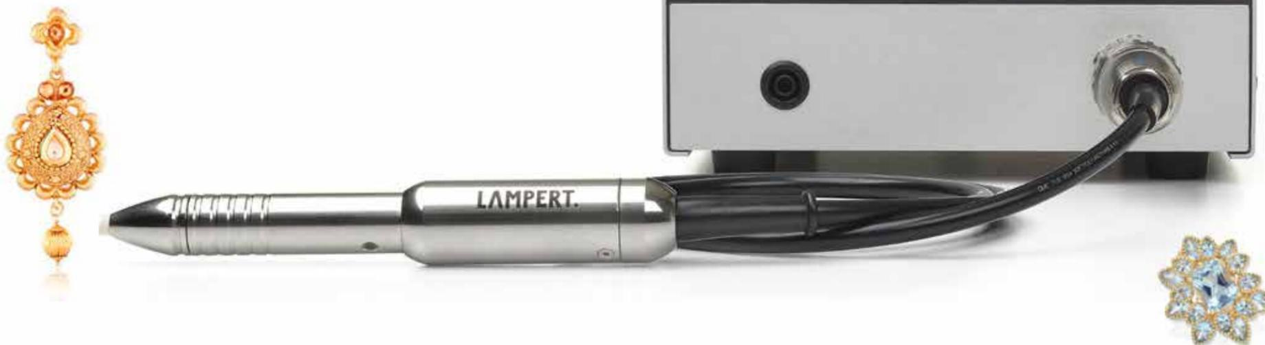
PUK welding's functional principle is as simple as it is ingenious. When the tip of the electrode in the welding handpiece touches the workpiece, the welding process starts automatically. Precisely on this touch point, an arc is ignited in an inert atmosphere as a lifting magnet in the handpiece withdraws the electrode.
