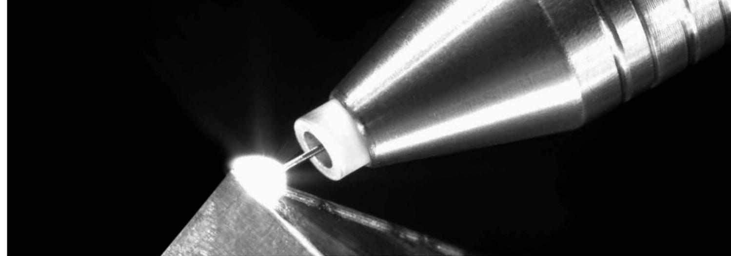
The PUK C140 precision welding device is a compact and versatile TIG impulse welder with which fine and minute welds can be carried out.
